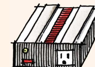
Inverter: Converts direct current (DC) energy to alternating current (AC) energy
